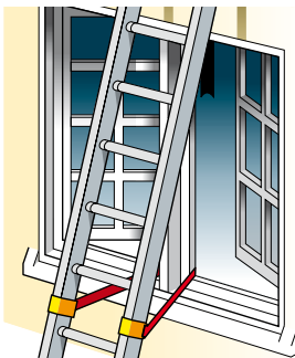
Figure 4 Ladder tied at top stiles (correct for working on, not for access)
